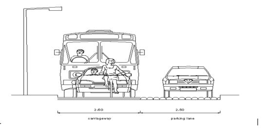
Traffic Management Layout Parameter Design Sheet establishes the guidance for the control and management of traffic at Roadworks Second Edition 2010. For a single lane/ shuttle the minimum width required is 2.5m to maximum 3.7m.
